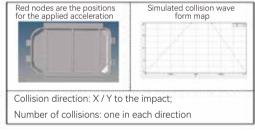
According to the national industry standard GB38031-2020, Pressler high-strength integrated battery tray, the collision simulation meets the standard.
