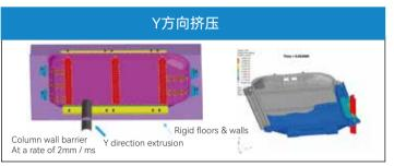
According to the national industry standard GB38031-2020, Pressler high-strength integrated battery tray, the collision simulation meets the standard.
