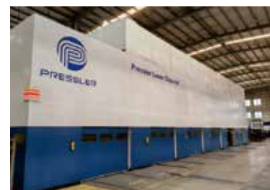
► Six-station laser cutting machine
