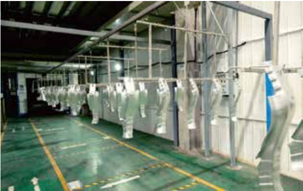
● Tempering line Size: 75m*4.7m*1.75m Capacity: 2.4 million pcs/year Speed of chain drives : 0.5m (1.2 hanger)/min, ≈10pcs/hanger
