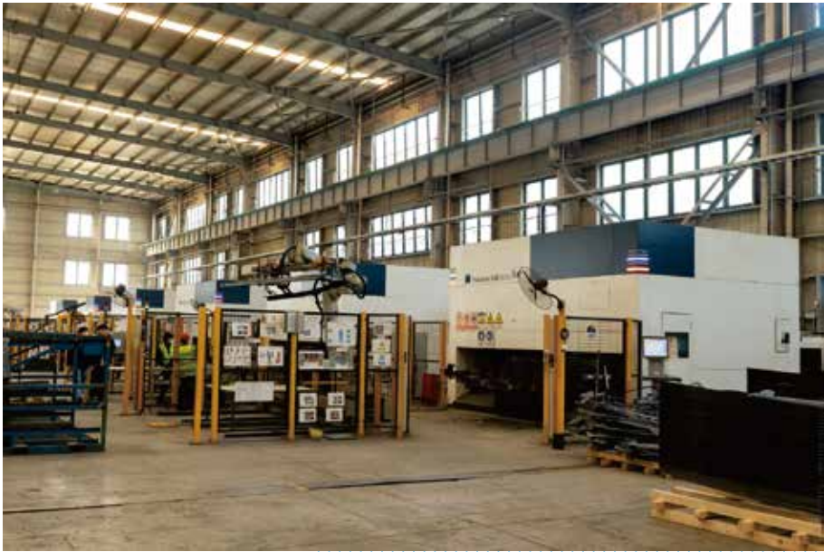
● Laser Manufacturer: TRUMPF/Pressler Table size: 2100*1600mm Laser-type : solid-state laser Note: Laser cutting ensures that all scrap is removed from each part (100% controlled). Maximum allowable burr ≤0.15mm.
