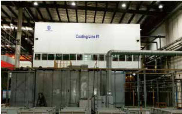
● Coating line Size: 100m*30m*8m Capacity: 2.4 million pcs/year Frequency: 30 flybar /3min
