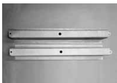
► 2000MPa Al-Si coated hot-formed parts
